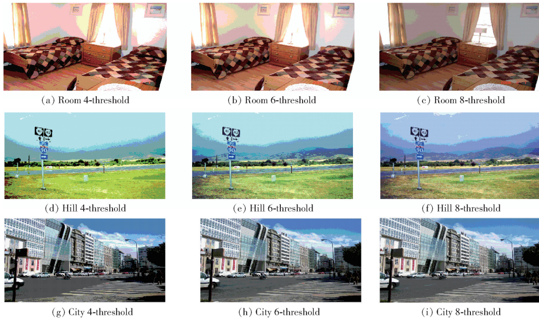
Fig. 6 Kapur-based multi-threshold segmentation results
