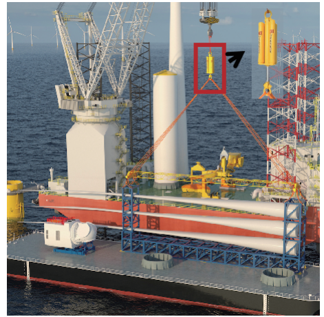
图 21 Cranemaster 公司从供给船向安装船吊装风电机组件 [58] Fig. 21 Cranemaster transferring wind turbine components from a supply vessel to an installation vessel [58]
