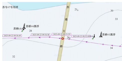
图 1 通过船舶 AIS 数据确定经过苏通大桥位置 Fig. 1 Determine the location of ships passing through the Sutong Bridge using AIS data
