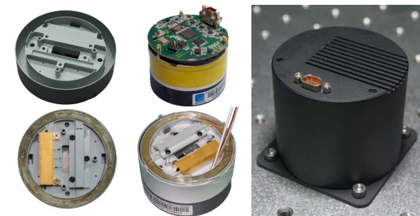
(a) 光纤骨架实物图 (b) 光路实物图 (c) 样机实物图 (a) Optical fiber (b) Fiber optic (c) Prototype physical carrier image structure image picture
