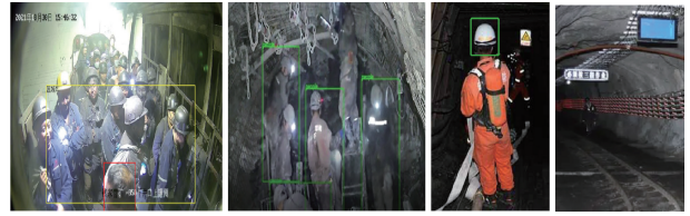
图 1 不同作业区域的安全帽佩戴识别 Fig. 1 Identification of helmet-wearing in different work areas
