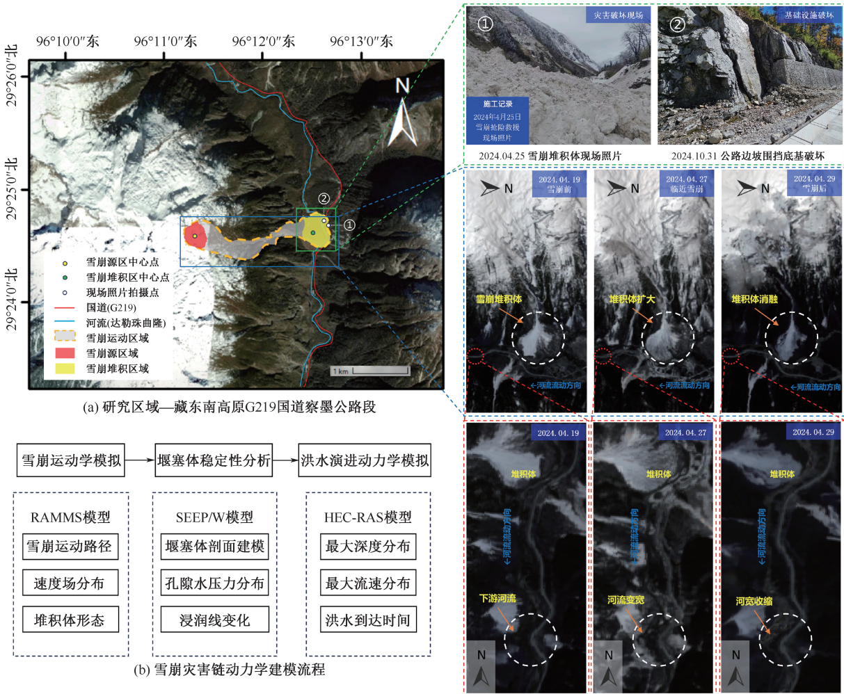
图 1 藏东南高原雪崩-堰塞湖-洪水灾害链动力学推演评估方法 Fig. 1 Dynamic deduction and evaluation method for avalanche-dammed lake-flood hazard chains in southeastern Tibet Plateau
