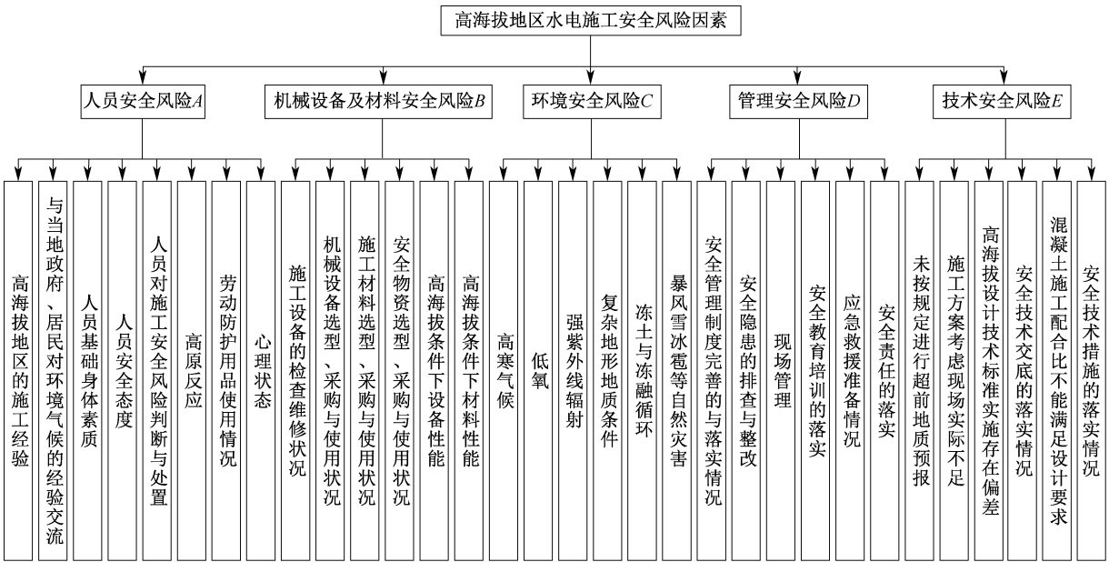
图 1 高海拔地区水电工程施工安全风险因素体系 Fig. 1 Construction safety risk factor system of hydropower projects in high-altitude areas
