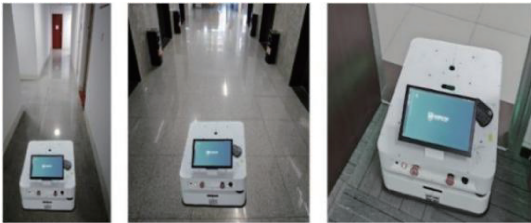
图 13 不同宽度狭窄道路真实试验场景 Fig. 13 Real experimental scene images of narrow roads with different widths
