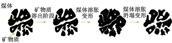
图 2 煤体在溶液浸泡过程中的变化 Fig. 2 Changes in the coal body during the immersion process in the solution
