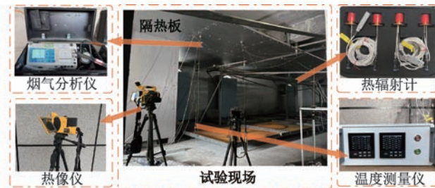
图 1 尺寸火灾燃烧特性试验测量系统 Fig. 1 Full-size fire combustion characteristic test measurement system
