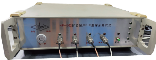
图 1 超声纵、横波测试仪 Fig.1 Ultrasonic P and S-wave tester
