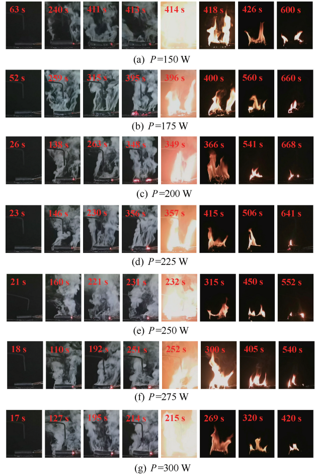
图3 内热源影响下电缆着火过程 ( S=35\text{ mm}^2 ) Fig. 3 Cable ignition process versus internal heat source power ( S=35\text{ mm}^2 )
