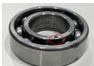
图 14 内圈磨损故障轴承 Fig. 14 Rolling bearing with inner ring wear fault
