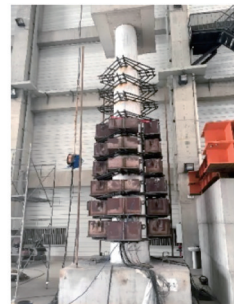
(c) 铁路圆端空心墩振动台试验 [14] (c) Shaking table tests of railroad round-end-shaped hollow pier [14]
