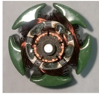
(a) 转子截面 (a) The cross section of rotor
