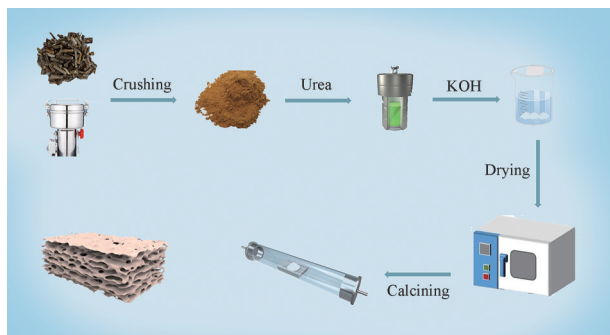
Figure 1 Scheme for preparation of 3DPC material. 3DPC: Three-dimensional ordered porous carbon materials
