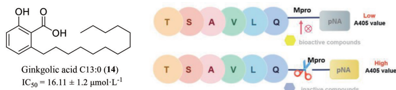
Figure 7 Schematic diagram of the colorimetric screening assay. The peptide (TSAVLQ-pNA) hydrolyzed by M pro has strong absorption at 405 nm and the solution turns yellow, the absorption at 405 nm is lower in the presence of bioactive compounds
