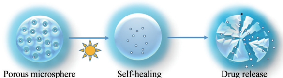
Figure 3 Schematic diagram of self-healing of porous microspheres. The surface pores of protein/peptide loaded porous polymers self-healing at a certain temperature and can slow down the drug release
