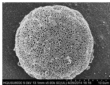
Figure 1 Scanning electron microscopy (SEM) image of poly(L-lactide) (PLLA) porous microspheres. (Quoted from Ref. 10. The image by Wang Y et al. is licensed under a Creative Commons Attribution 4.0 International License, no change from original). The PLLA porous microspheres was prepared in a high-voltage electrostatic anti-solvent process with the geometric diameter ( D_g ) is 19.1 \pm 0.4 \mu\text{m} , the density is 0.289 \pm 0.004 \text{ g}\cdot\text{cm}^{-3} and the aerodynamic diameter ( D_a ) is 4.2 \pm 0.2 \mu\text{m}
