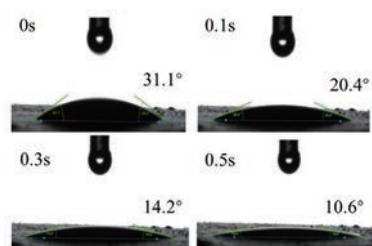
Figure 10 Dynamic diagram of the contact angles of the determined printing ink with the powder
