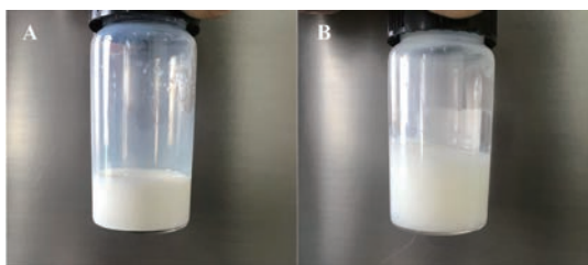
Figure 1 Appearance of fluorocarbon microemulsion (FM, A) and fluorocarbon microemulsion-based gel (FMBG, B)
