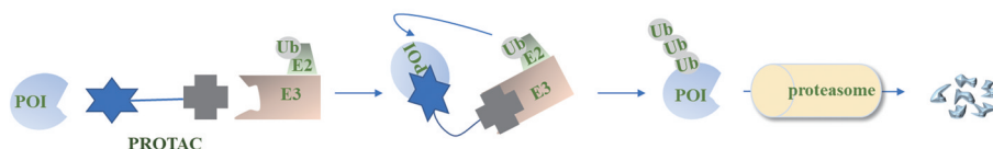
Figure 6 Mechanism of proteolytic targeting chimera (PROTAC)-mediated protein degradation
