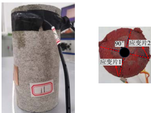
图 3 贴应变片 Fig.3 Attaching strain gauges
