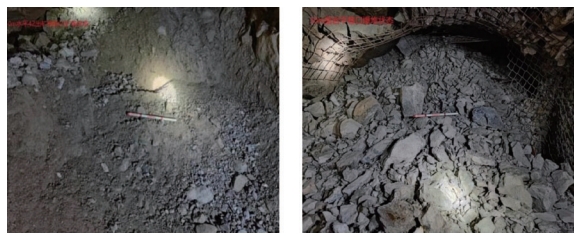
Fig. 13 Muck pile condition with 65 mm blast holes at draw point
