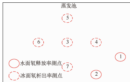
图 2 蒸发池氡释放率布点示意图 Fig. 2 Sketch diagram of monitoring points distribution of radon release rate on evaporation pond
