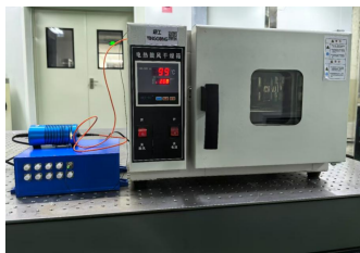
图4 金涂覆光纤传输损耗测试系统 Fig. 4 Gold-coated fiber transmission loss test system
