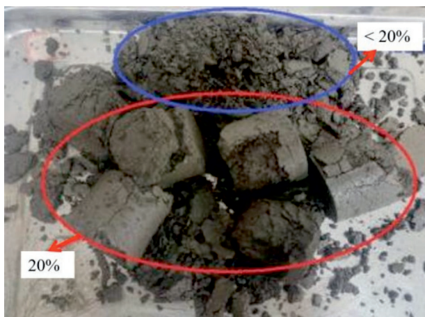
Fig. 11. Compression failure morphology of specimens.
