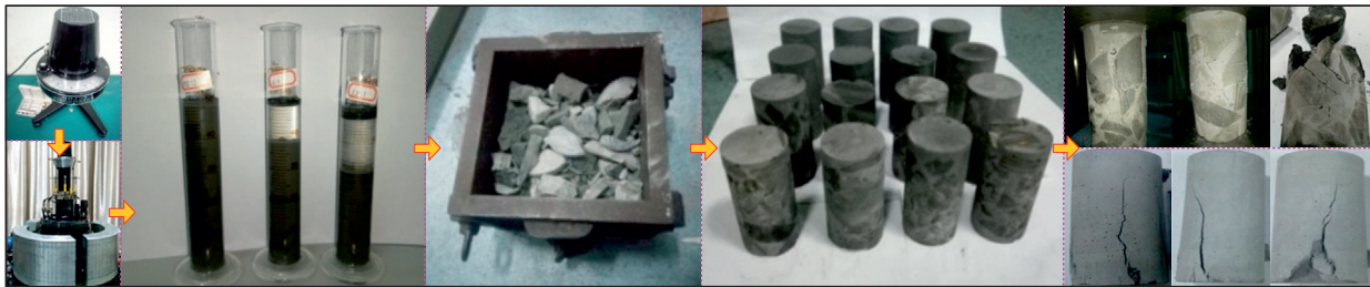
Fig. 27. Failure test of grouting reinforcement rock.
