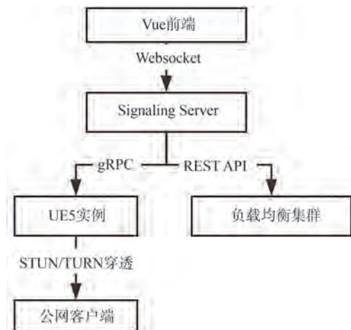
图3 系统像素流送架构 Fig. 3 System pixel streaming architecture
