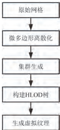
图2 HLOD代理模型生成逻辑 Fig. 2 Generation logic of HLOD proxy model
