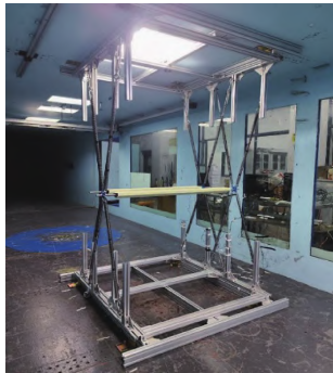
图 2 双主缆节段模型测振风洞试验照片 Fig. 2 Segmental model of dual main cables in the wind tunnel test
