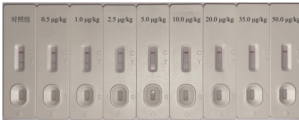
图 5 啶虫脒的标准曲线的测定 Fig.5 Determination of the standard curve of acetamiprid
