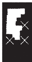
图 2 交叉多裂隙岩体单轴压缩 PFC 数值模型 ( \alpha = 90^\circ ) Fig. 2 PFC2D numerical model for uniaxial compression of intersecting multi fractured rock masses ( \alpha = 90^\circ )
