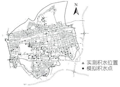
图 2 模拟积水位置与实测积水位置对比 Fig. 2 Comparison of simulated water accumulation location and measured water accumulation location
