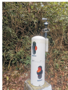
图 1 跨屋溪蠕变体典型监测点便携式气象站安装 Fig. 1 Installation of a portable meteorological station at a typical monitoring point
