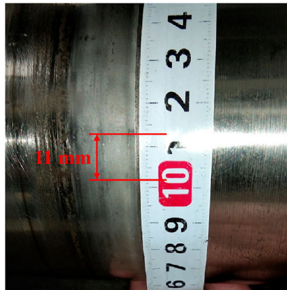
Figure 12. Corrugation wavelength for condition 4. Source: Authors' own work
