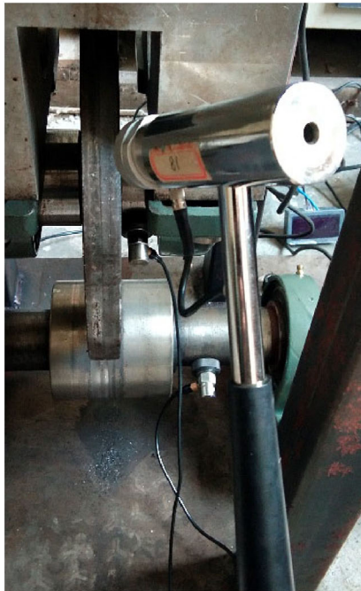
Figure 10. The percussion hammer. Source: Authors' own work
