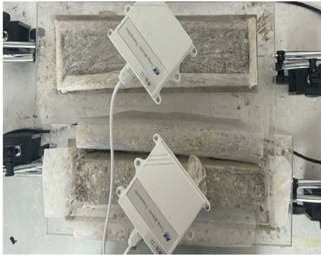
Figure 3. Shrinkage and humidity test specimens. Source(s): Authors' own work
