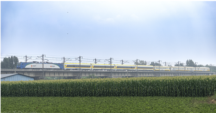
Figure 2. Intelligent heavy-haul comprehensive inspection vehicle. Source(s): Authors' own work
