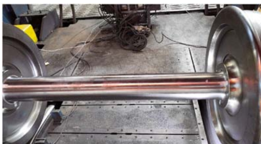
Figure 14. Wheel set with a damping ring and overall constrained damping structure. Source: Authors' own work
