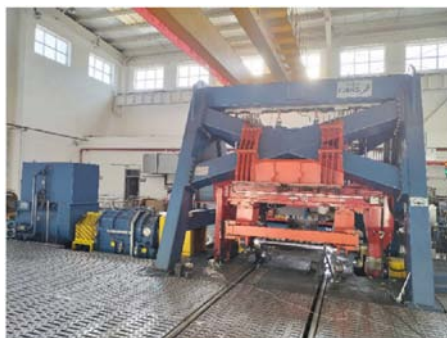
Figure 7. High speed wheel–rail relationship test bench test. Source: Authors' own work
