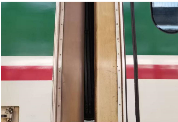
Figure 1. Yellowing of windshield rubber. Source(s): Author's own work
