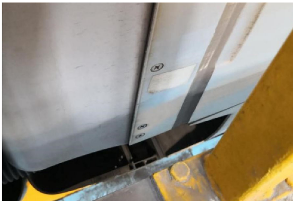
Figure 4. Adhesive tape application. Source(s): Author’s own work
