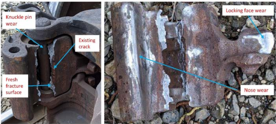
Figure 3. Failed knuckle, intact with the coupler system, and in isolated condition. Source(s): Reddit, ( Justrolledintotheshop, 2019 ), with permission
