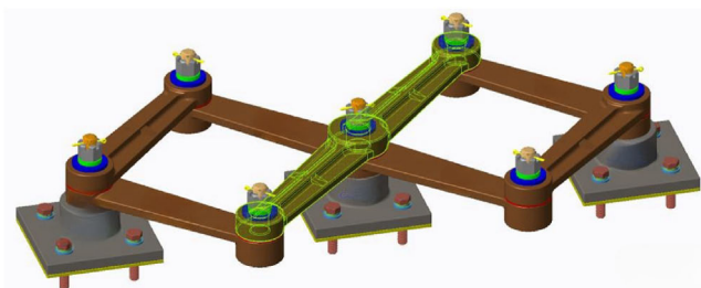
Figure 11. Detailed design of scissor mechanisms for deck-type BEJ
