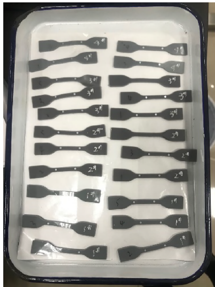
Figure 1. Samples of 7 different components before and after ultraviolet aging. Source: Author's own work
