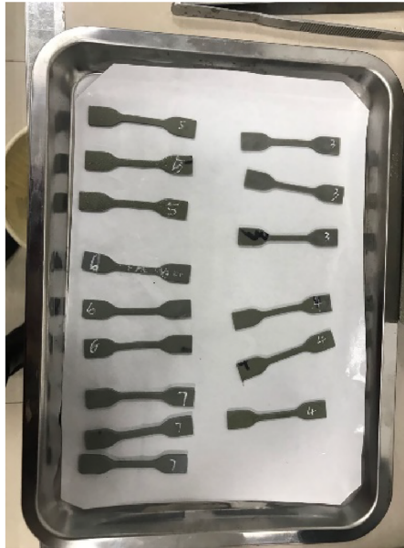
Figure 2. Samples of seven different components before UV aging. Source: Author's own work
