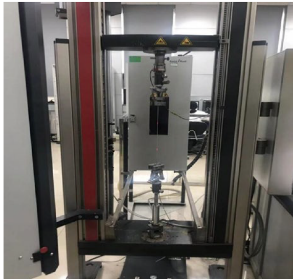
Figure 3. Zwick high and low temperature electronic universal material testing machine. Source: Author's own work
