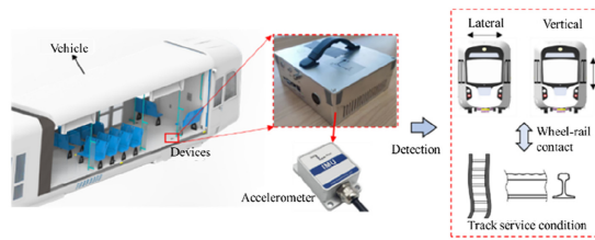
Schematic of the condition monitoring of the vehicle-track system by sensing terminal
