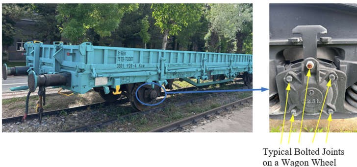
Figure 1. Schematic representation of a bolted rail-wheel joint. Authors' own work
