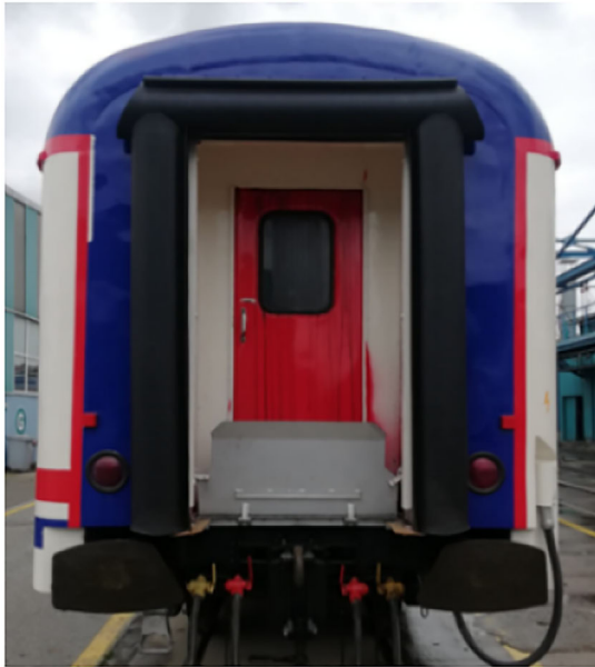
Figure 2. Front/rear mask for wagon. Source: Authors' own work
