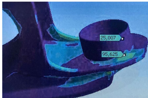
Figure 13. Stresses on the edge of the spring box in the bed box. Source: Author’s own work
