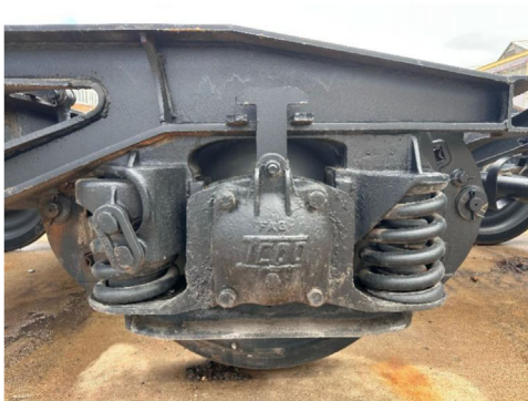
Figure 4. The general primary suspension system. Source: Author's own work
