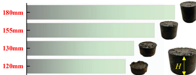
Figure 15. Initial HRGA fillers thickness ( H_0 ). Source(s): Authors' own work
