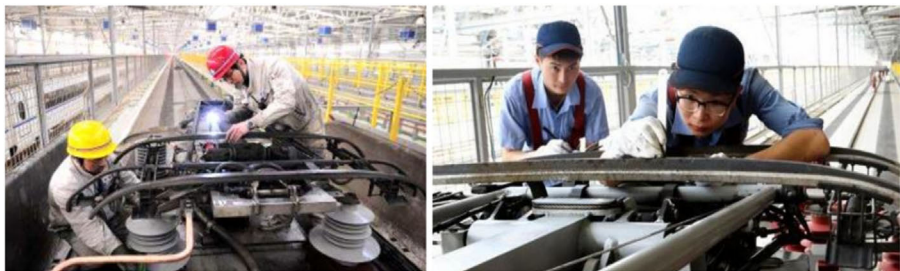
Figure 7. Technicians measuring wear on the CS. Source(s): Lu et al. (2021)
