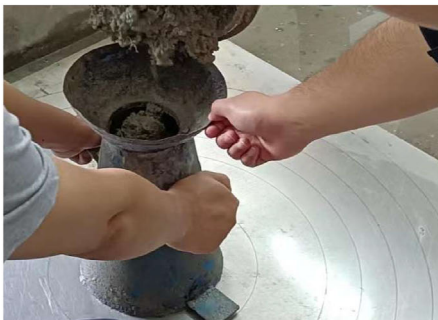
Slump bucket and measuring platform
