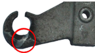
Figure 15. Wear and failure of positioning hook. Source(s): Authors' own work
